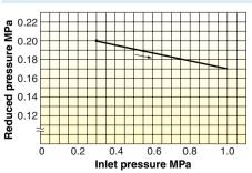
This chart shows variation in reduced pressure when the inlet pressure of 0.3 MPa is changed between 0.3 MPa and 1.0 MPa while the reduced pressure is set at 0.2 MPa.
