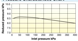
This chart shows variation in reduced pressure when the inlet pressure of 400 kPa is changed to 10 kPa while the reduced pressure is set at 8.0 kPa.
