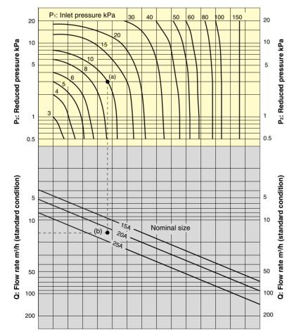
Table 1: When the inlet pressure is between 200 kPa and 400 kPa
