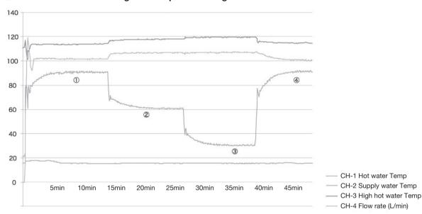
Setting condition Supply water: 18 degrees C Setting of hot water temperature: ①90 degrees C, ②60 degrees C, ③30 degrees C, ④90 degrees C High hot water temperature: 120 degrees C Setting of hot water flow rate: At the stage of 1, fixing 100 L/min by manual valve
